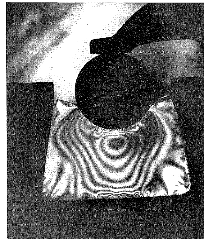
▼ Figure 4—Sheave Liner—Actual Stress Pattern.
