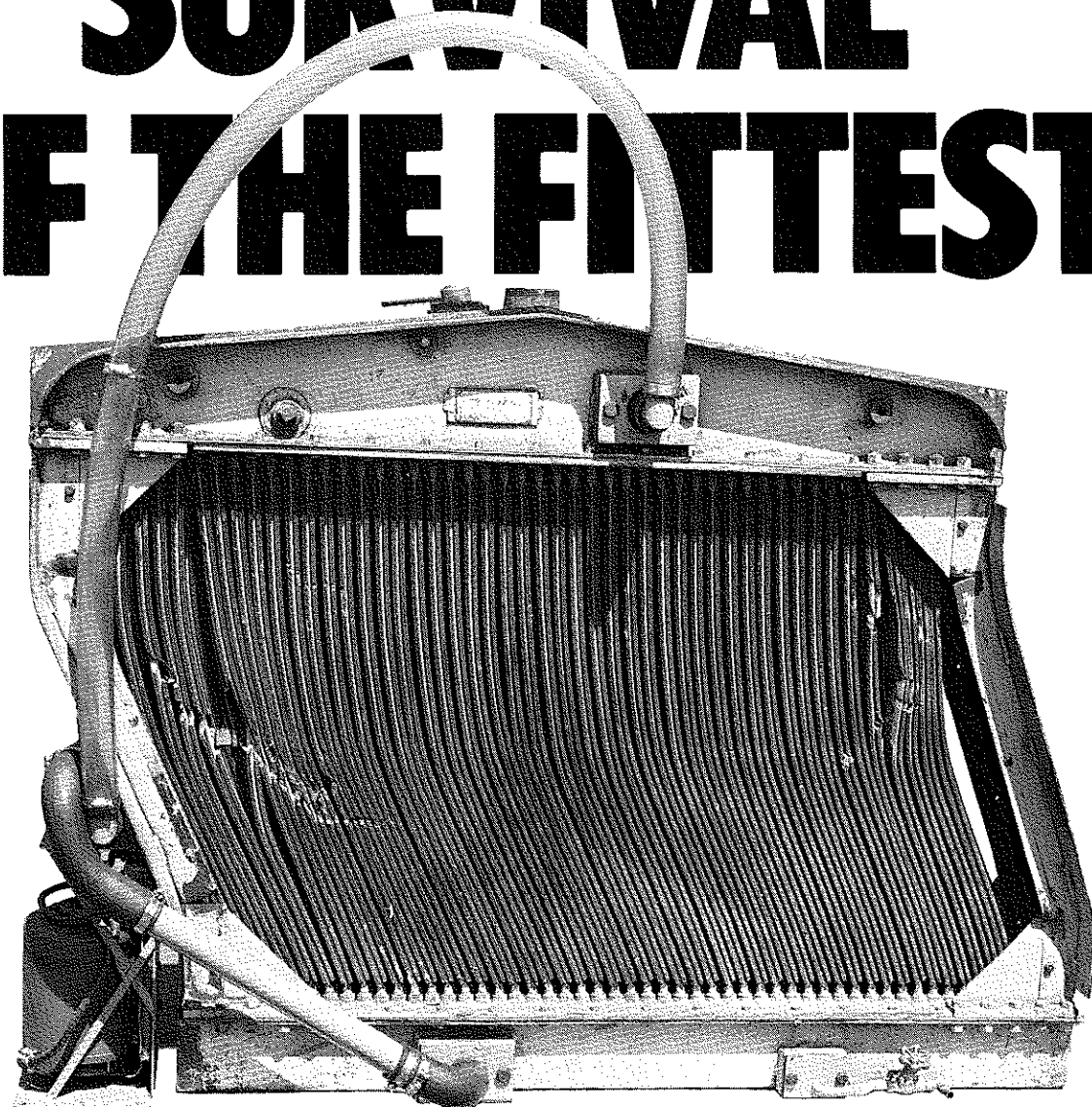
Although bent into a figure "S" as a result of a truck rollover, this MESABI Core Radiator refuses to leak. As the only workable component salvaged from the truck, the core has been fitted with an electric water pump and makes a regular circuit of trade shows to demonstrate the reliability of the MESABI Core Radiator.
