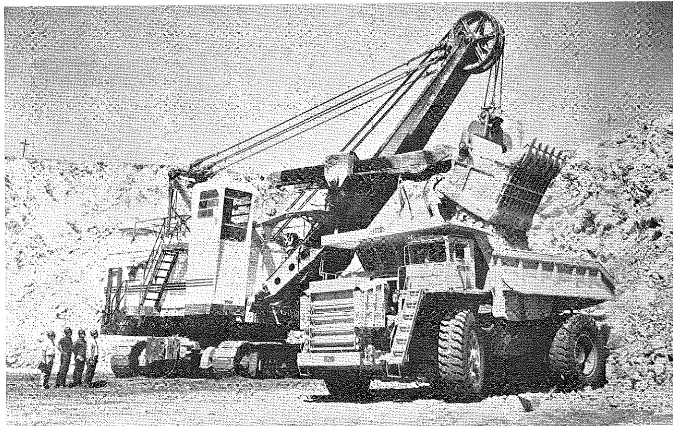
POWER SHOVEL BUCKET drops approximately 23 tons of copper-molybdenum ore into 1000 HP haul truck. When fully loaded, the haul truck will carry 120 tons of ore. Each truck tire is 48-ply, stands nine feet high and weighs 3000 pounds.
