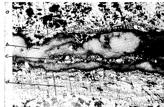
▼ Figure 2. Mineral Material in Coal: a. Semifusinite; b. Calcite; c. Pyrite; d. Narrow band of Vitrinite.
