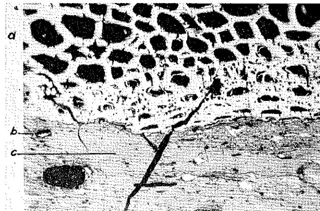
Figure 4. Fusinite: a. Typical course cell structure frequently found in fusinite; b. Small bituminous body; c. Vitrinite with small white inclusions of micronite.
