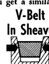
It's the sides of a V-Belt that do all the gripping and get all the wear. That's why longer life for the sides means longer life for the belt.
