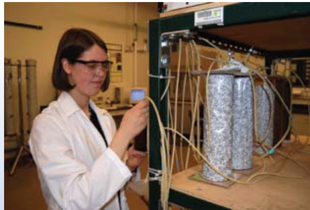
Clockwise from top left: AQWATEC staff, Dr. Chris Belton and John Luna, reload a nanofiltration membrane into a pilot-scale skid at a water reuse facility in California. Gretchen Oldham, a graduate research assistant, simulates the mechanisms of riverbank filtration in small-scale column systems. Nathan Hancock, a doctoral student, and Professor Tzahi Cath adjust a 1,000 gallon tank that is used to provide water to pilot-scale membrane units.
