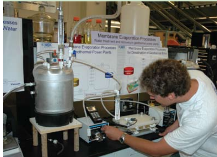
Nathan Walker, a graduate research assistant, is testing membrane distillation as a novel process to treat brine from geothermal power plants.
